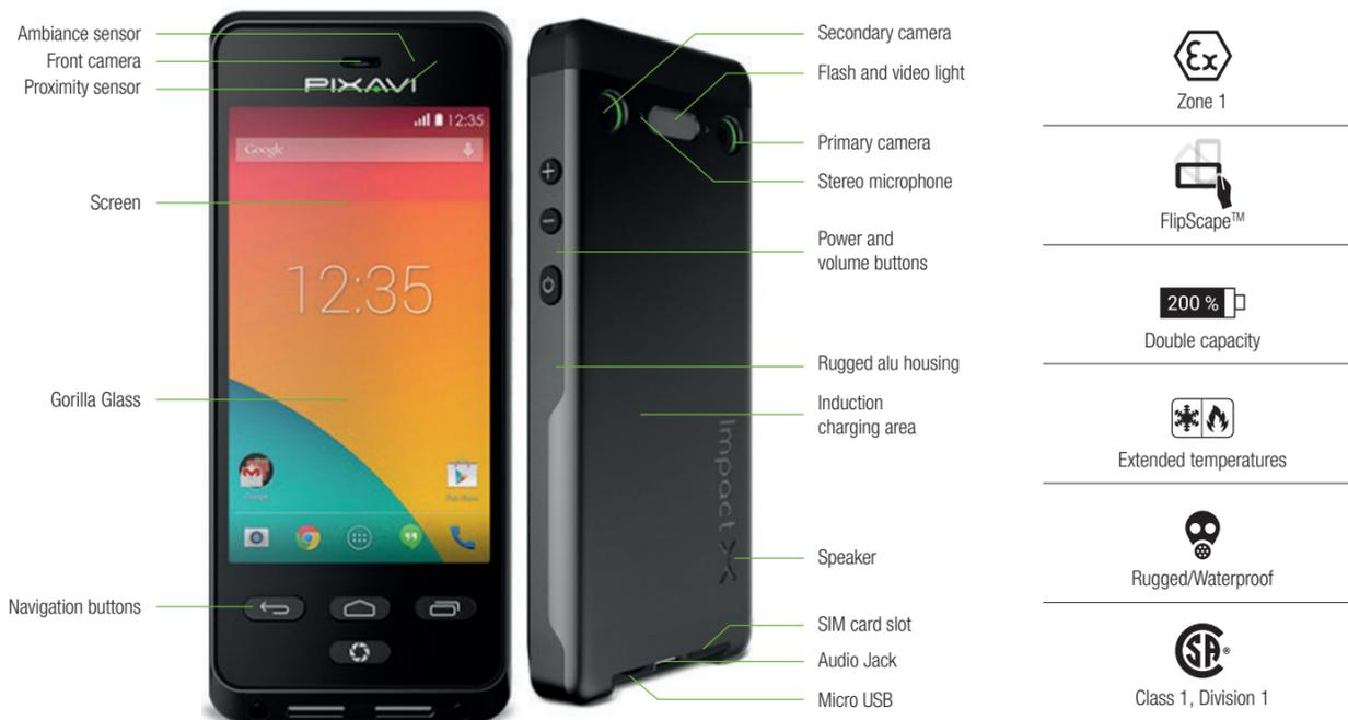
The BARTEC PIXAVI Impact X is the toughest smartphone you will ever meet. This intrinsically safe smartphone has all the functionality you will expect from a regular smartphone. The CSA, IECEx and ATEX certification has not compromised the quality and usability. The device is explosion-proof and certified for use in hazardous areas. The Impact X is the next generation wireless video communication technology from BARTEC PIXAVI.
